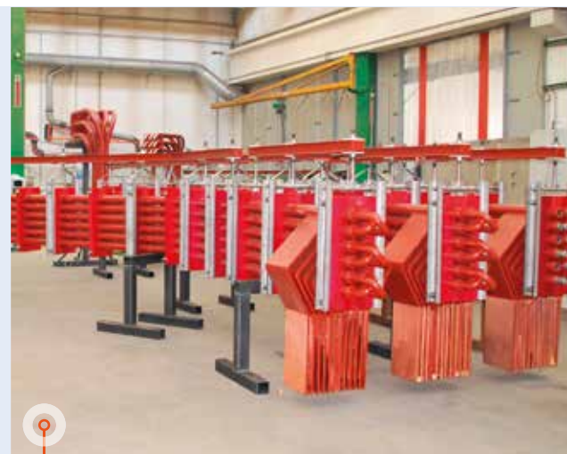
Circuito secondario raffreddato per forno SAF / Cooled secondary circuit for submerged arc furnace
