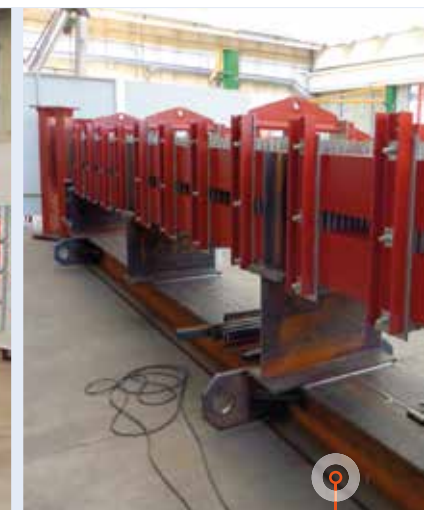
Circuito secondario a barre per forno SAF / Secondary circuit with rectifiers for submerged arc furnace
