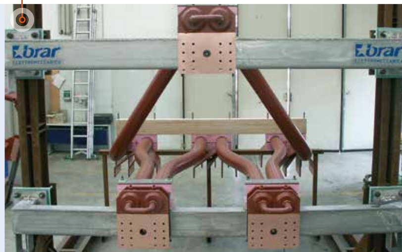
Circuito secondario con chiusura del triangolo / Secondary circuit with closure of the triangle
