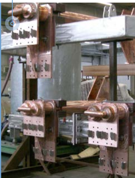
Aggancio rapido lato secondario / Quick coupling on the secondary side
