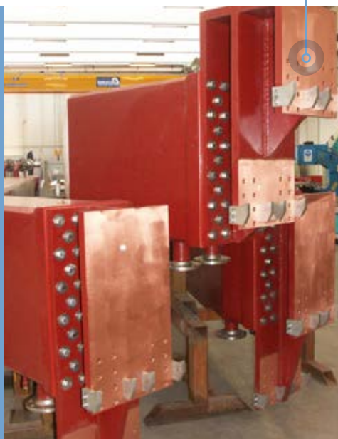
Aggancio rapido lato bracci / Quick coupling on the arm side
