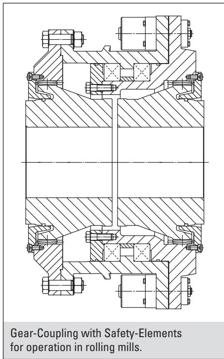
Gear-Coupling with Safety-Elements
